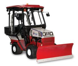
Ventrac KD Power Angle Dozer Blades have working widths of 48, 60, and 72 inches (122, 152, and 183 cm). All control functions are performed with the S.D.L.A. Control for raising and lowering the blade or angling it left or right. Adjustable cast iron skid shoes accommodate dozing at selected heights, such as moving snow on gravel driveways.
