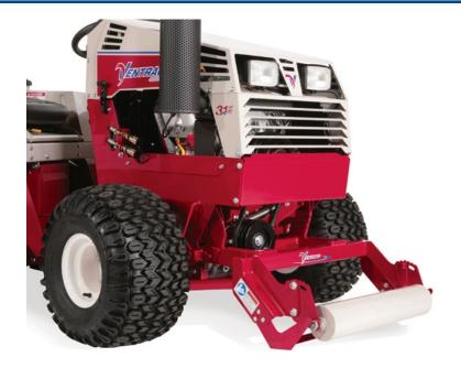
Ideal for landscapers or homeowners, the EC240 sod cutter cleanly cuts sod for flowerbeds, walkways, and lawns. With a cutting depth of 0 to 2  $\frac{1}{2}$  inches, the EC240 can be used to cut thick lush grass or even to shave off the last bit of dirt to prepare your work site.
