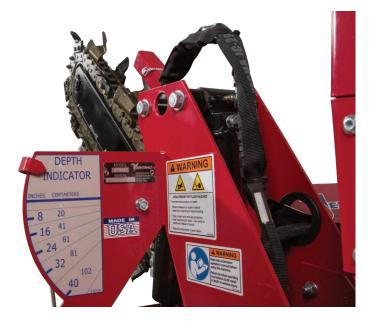
The KY400 Trencher is capable of trenching up to 40 inches (102cm) in depth with a 5½-inch (14cm) wide cut. It is designed with dual Push-N-Pull cylinders to assure positive boom control for digging, boom lift, and transport.
